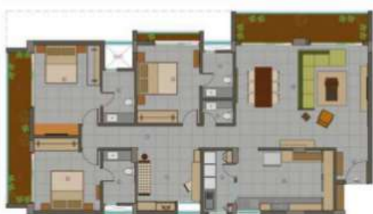
A-Foyer, B-Living room/dining area, C-Balcony, D-Kitchen area, E-Utility area, F-Public toilet, G-Att. toilet, H-Bed room-1, I-Wash area, J-Study room, K-Master bedroom-1/2.
